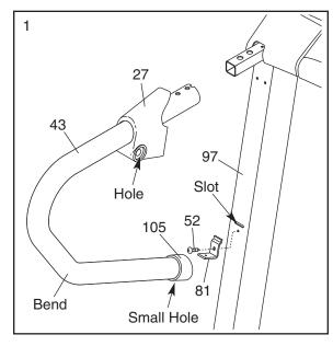
Slide the left Handrail (43) onto the post on the left Upright (97) and onto the left Handrail Bracket (81). Finger tighten two Handrail Bolts (80) into the left Handrail and the post; do not fully tighten the Handrail Bolts yet.
